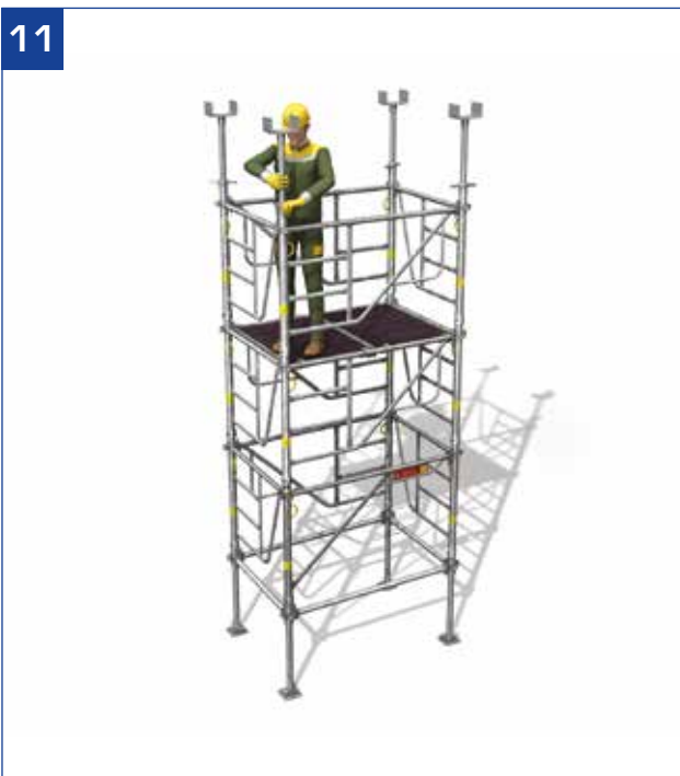
- Set up and adjust the head jacks.
