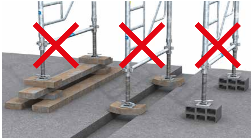
Excessive chock stacking
